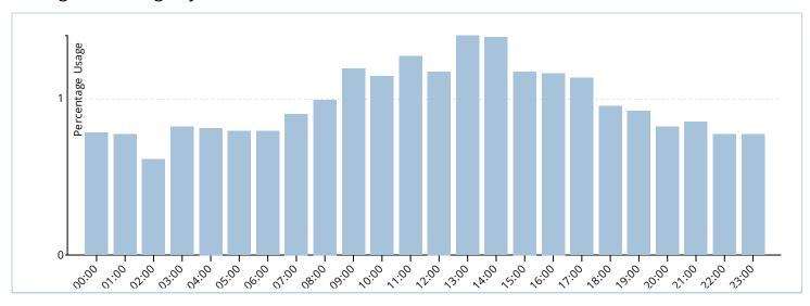
Similarly, memory usage over time is an indicator of the FortiGate's sustainability in the target network environment. memory usage may remain high even when throughput is relatively low due to logging activity (or queued logging activity) over time.
