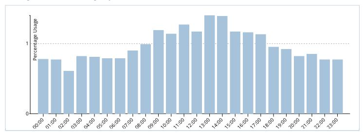
Session averages on a daily basis are useful for calculating throughput and proper sizing. It can help when determining peak planning as a typical enterprise will see more sessions being generated in the morning when the network is at its most active.
